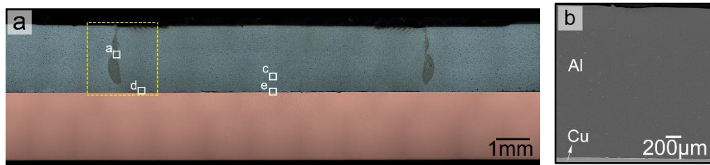
Figure 5.17 Typical Al/Cu friction spot-welded joint: (a) cross section of the as-etched sample, the four white boxes indicate the region for SEM analyses in Figure 5.19; (b) back-scattered image from the as-polished sample, it was taken from the location marked with a yellow dashed box in (a). Welding condition: RS = 1200 rpm, PD = 1.6 mm, DT = 0.
