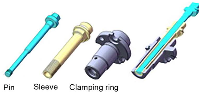
Figure 3.3 Schematic illustration of the three-piece tool system used in the FSpW process [28].
