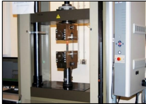
Figure 4.4 Machine Zwick/Roell used for lap-shear test.
