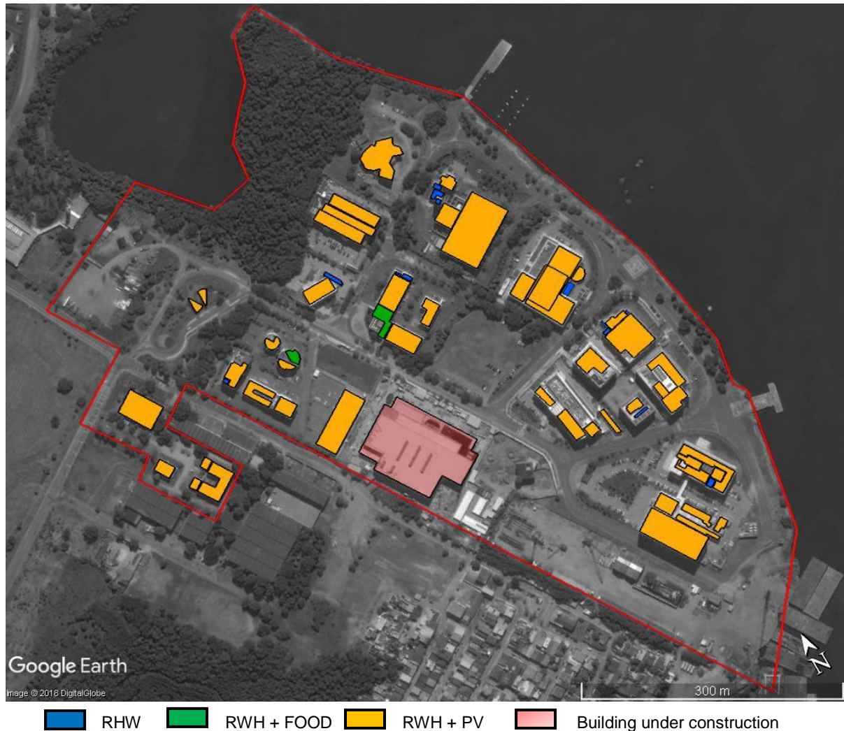
Figure 7.4. UFRJ Technology Park with Roof Mosaic
