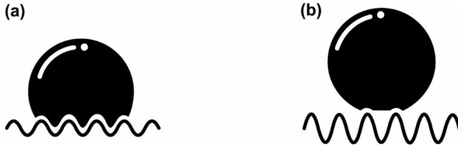
Figure 3.4 - Wetting models proposed by (a) Wenzel and (b) Cassie-Baxter
