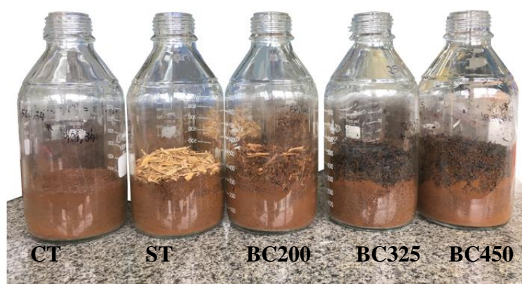
Figure 13. Microcosms with the samples of soil (CT), soil + in natura sugarcane trash (ST), soil + biochar 200 °C (BC200), soil + biochar 325 °C (BC325), soil + biochar 450 °C (BC450).
