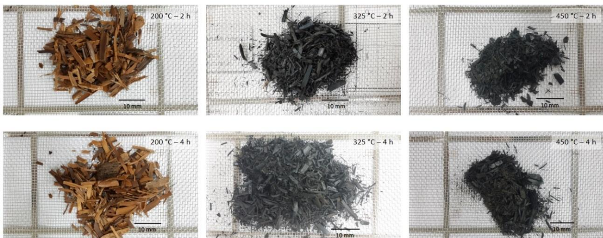
Figure 4. Biochar produced by different conditions: 200 °C/2h, 200 °C/4h, 325 °C/2h, 325 °C/4h, 450 °C/2h and 450 °C/4h.
