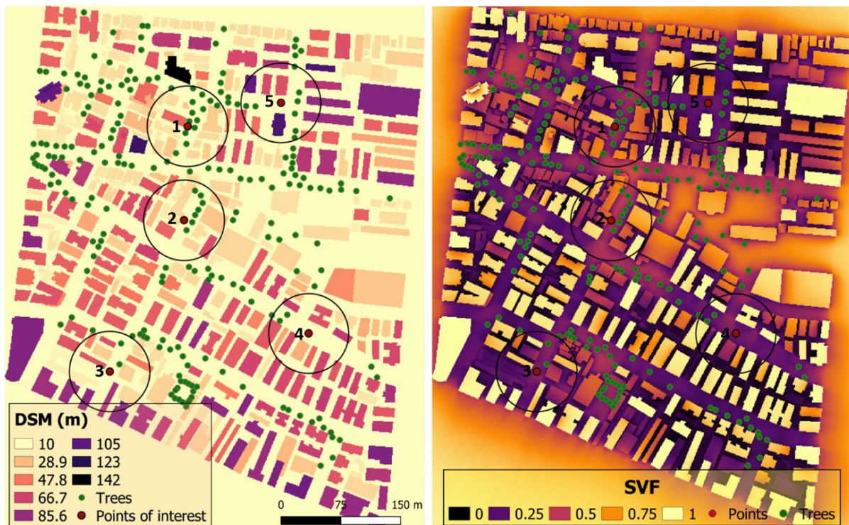
Figure 34. Urban morphology featured in HRB. Highlight for building digital surface model (DSM) (left), SVF (right), trees, and points of interest (used PET calculations).
