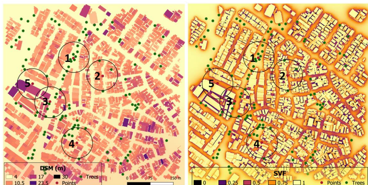
Figure 35. Urban morphology featured in CLR. Highlight for building digital surface model (DSM) (left), SVF (right), trees, and points of interest (used for PET calculations).
