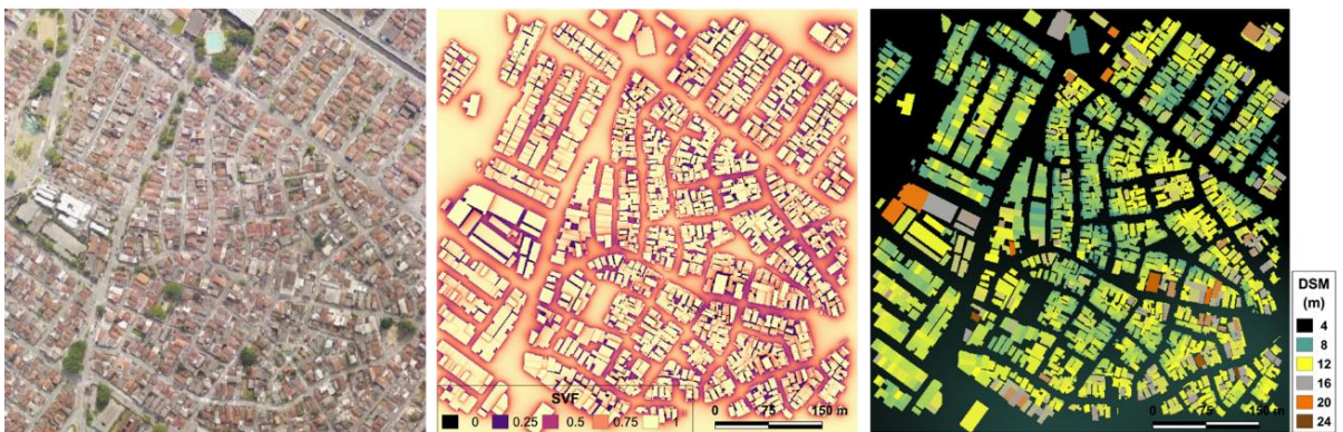
Figure 24. Screenshots from Google Earth (left), SVF (middle) and digital surface model (right) of the compact low-rise building (CLR2). Differences between the image and the models are related to the date of acquisition of each product (satellite images are more recent).
