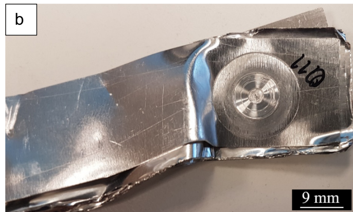
Figure 5.1 – Representation of welds (a) that bonded to the backing and (b) with twisted materials.
