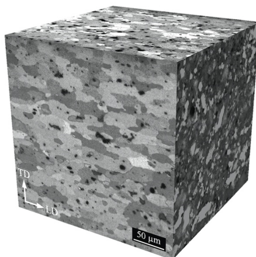
Figure 4.1 – 3D microstructure of the AA2024 base material. Credit to the author.
