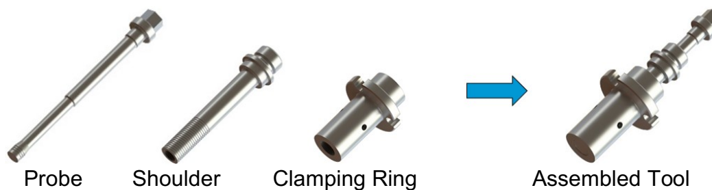
Figure 3 - Refill Friction Stir Spot Welding tool pieces and assembly.
