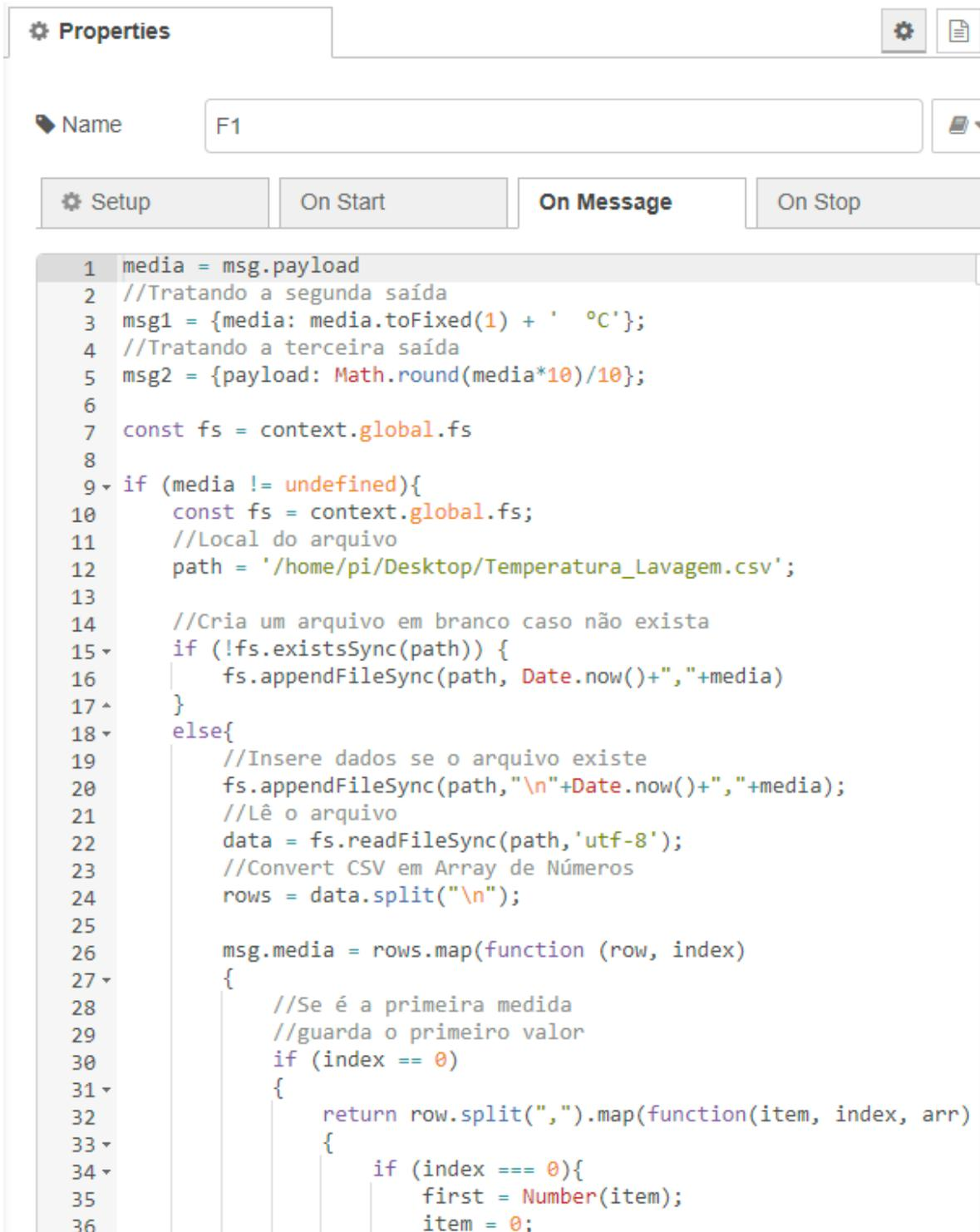
The image shows a screenshot of a Node-RED function node configuration. The node is named 'F1'. The 'On Message' tab is selected, showing the following JavaScript code:
