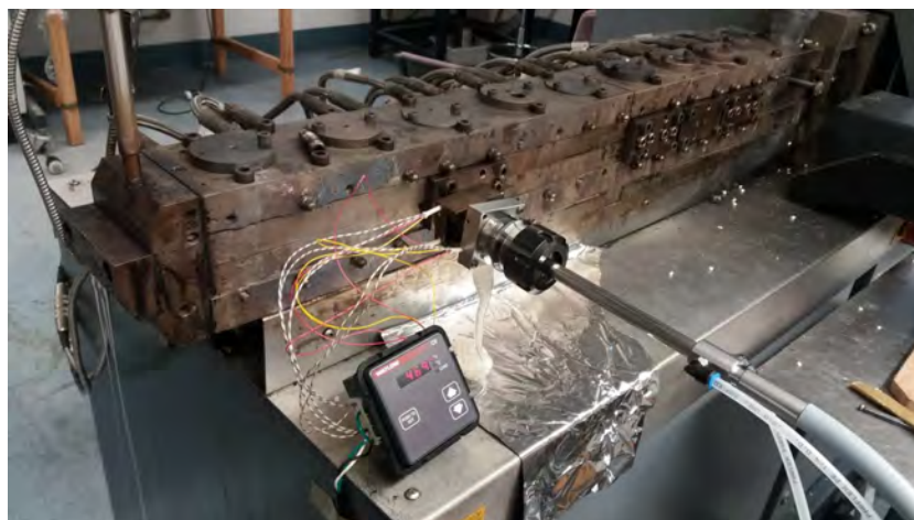
Figura 7.1: On-line FTIR system attached to the extruder. In the picture the temperature control system, the PHU, the air cooling system and the ATR-FTIR probe is shown
