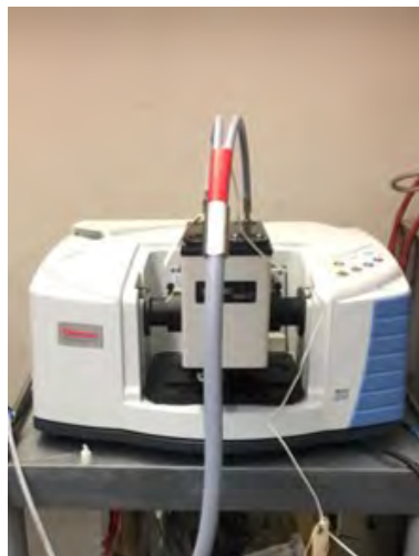
Figura 7.3: Nicolet IS 10 MID (4000 to 400 \text{cm}^{-1} ) infrared spectrometer (ThermoFisher Scientific).
