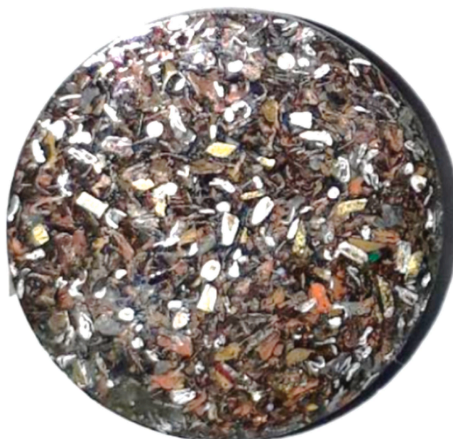
Fig. 2. Sample immobilized in epoxy resin after the sanding and polishing step. Each piece was approximately 25 and 20 mm in diameter and high, respectively.
