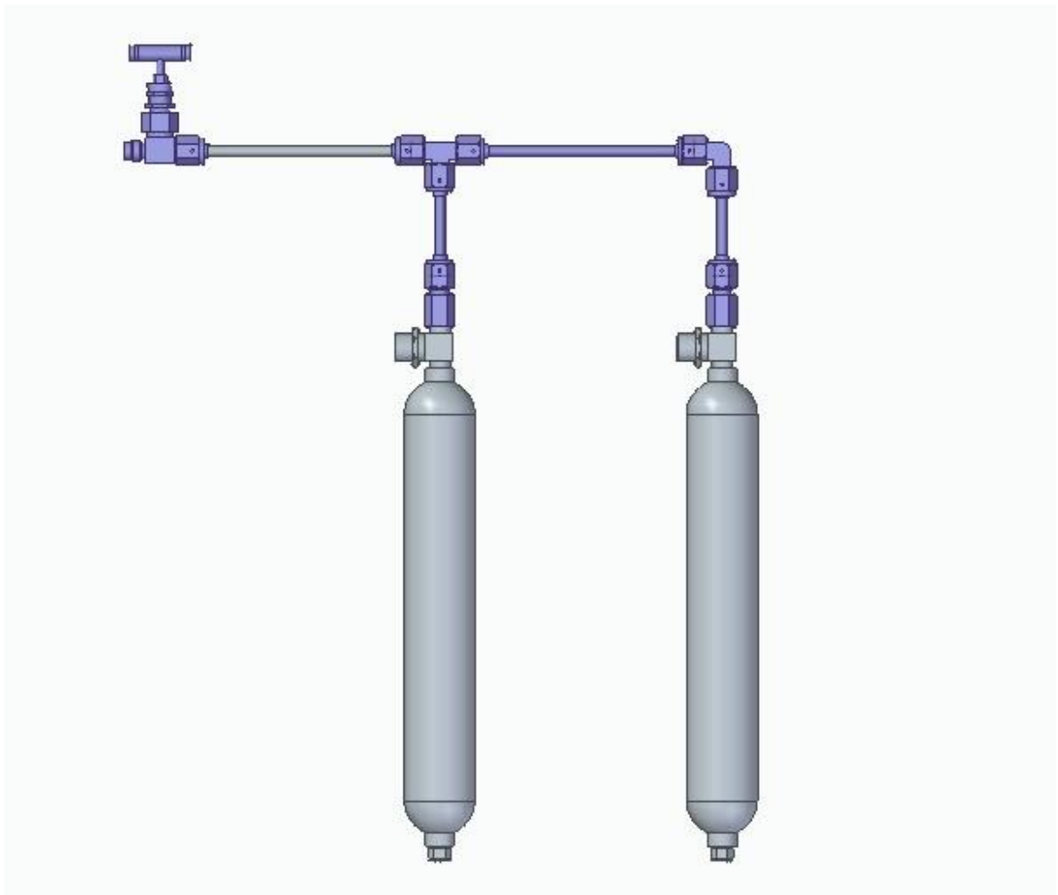
Figure 10: 3D drawing of project A, with two sample cylinders of 500cm 3 .
