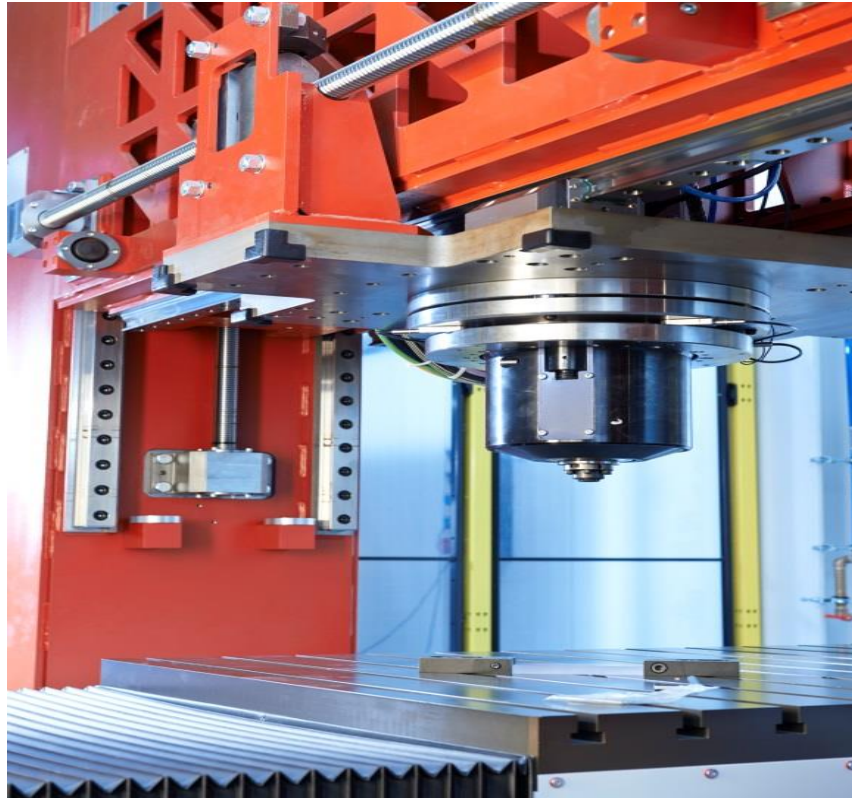
Figure 7: Automated RSM 410 welding system for the production of friction-riveted joints (image source: Hereon).
