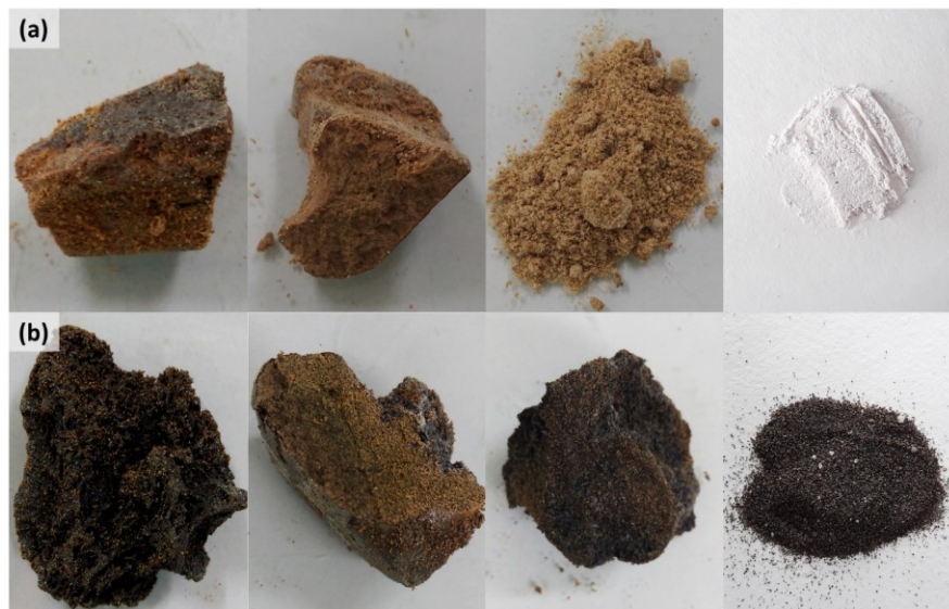
FIGURE B1. (a) From left to right: PolyS-Str25, PolyS-Str50, PolyS-Str75 and pure struvite; (b) From left to right: PolyS-Bay25, PolyS-Bay50, PolyS-Bay75 and pure Bayóvar rock.
