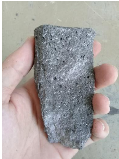
Figure 87: UHPC inner bubbles in specimen with 4% superplasticizer
