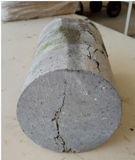
Figure 104: Failure mode of UHPC splitting test: (a) specimen front at 7 days, (b) specimen back at 7 days, (c) specimen front at 28 days, and (d) specimen back at 28 days
