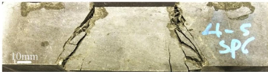
Figure 55: Cracking behavior of UHPC during the shear test
