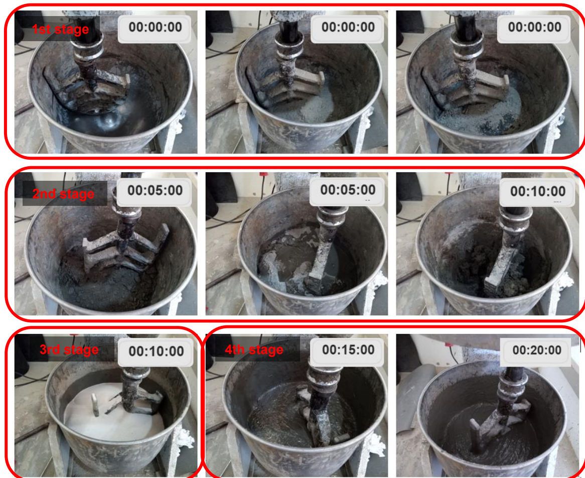
Figure 71: Four-stage UHPC mixture sequence
