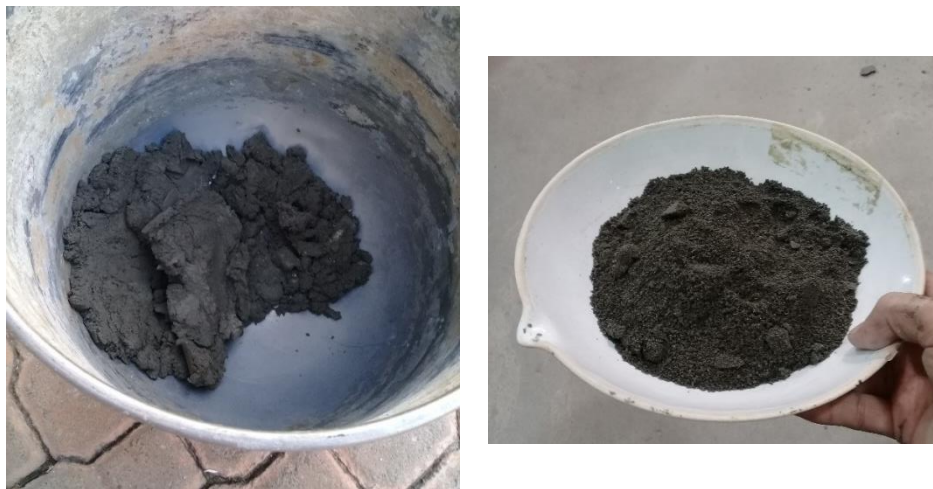
Figure 70: Poor fluidity in three-stage mixture UHPC
