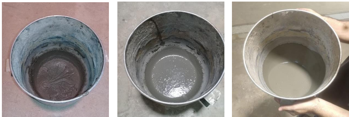
Figure 67: Progressive development of UHPC consistencies
