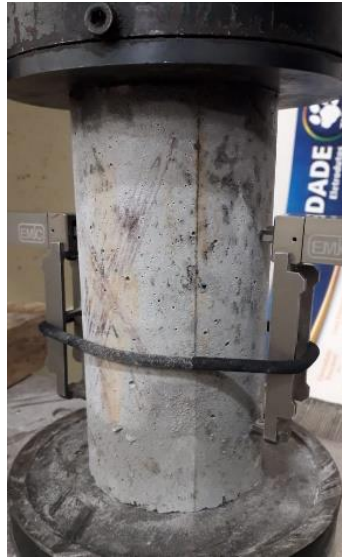
Figure 75: The elasticity modulus test setup
