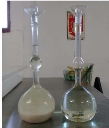
Figure 66: Quartz powder-specific density test
