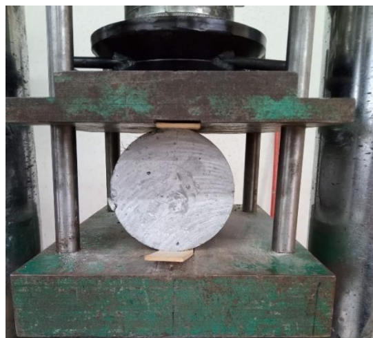
Figure 76: Tensile splitting test setup
