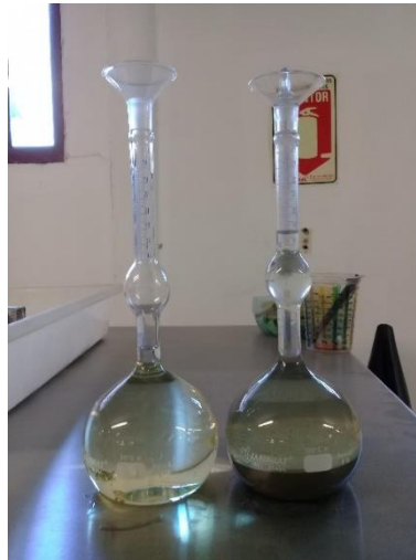
Figure 61: Cement-specific density test
