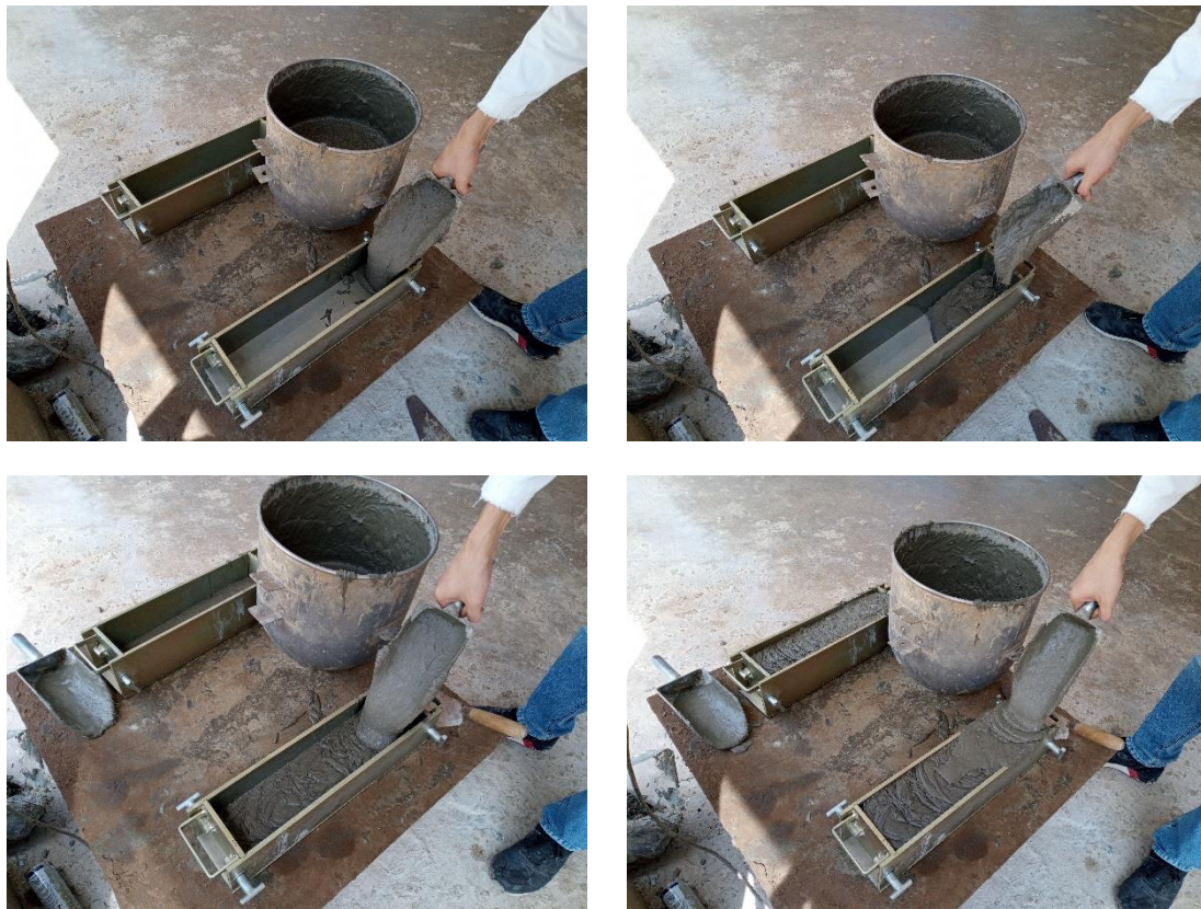
Figure 72: UHPC prism placement sequence
