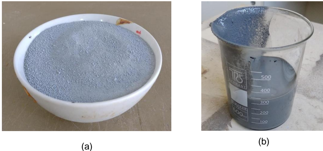
Figure 62: SF in (a) a dry state and (b) an aqueous medium
