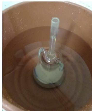
Figure 64: Sand-specific density test
