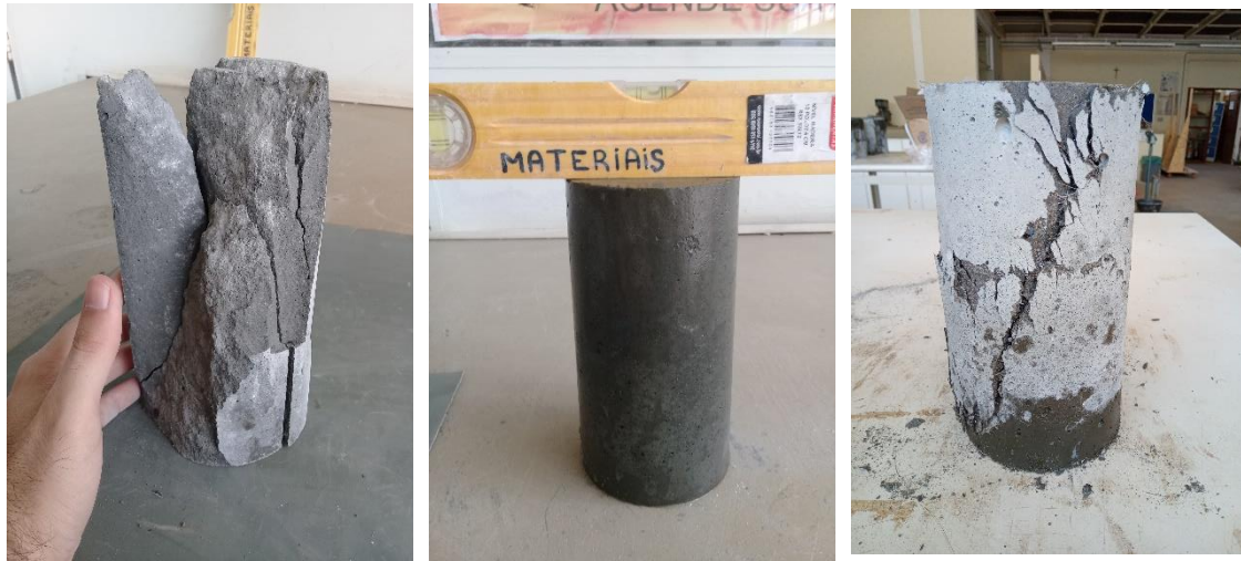
Figure 92: UHPC 10 × 20 cm ruptured specimens: (a) without fibers, (b) top surface level verification, and (c) with fibers
