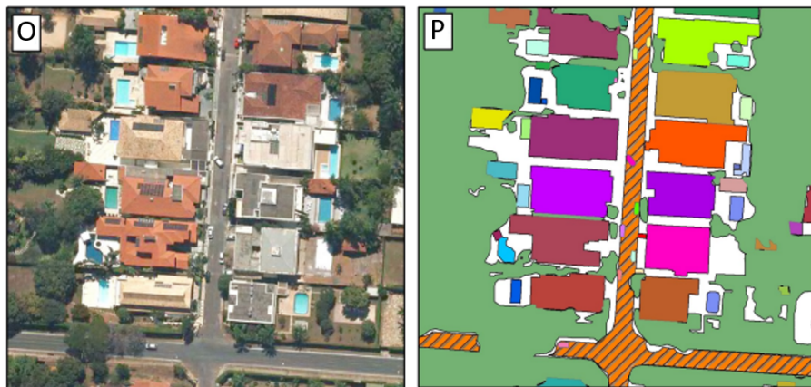
Figure 18 – Panoptic segmentation example. The original image is on the left, and the segmented output is on the right. Source: Carvalho et al. (2021) .
