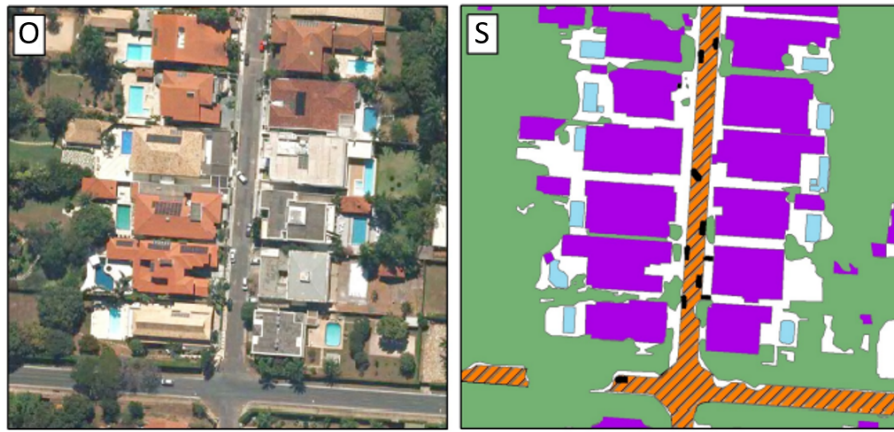
Figure 16 – Semantic segmentation sample with the original image on the left and segmented output on the right. Source: Carvalho et al. (2021).
