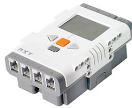
Figura 2.6: Brick NXT da LEGO Mindstorms (KNUTH, 2011)
