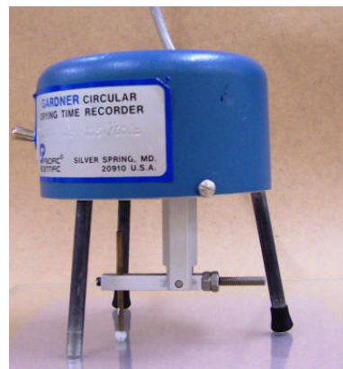
Figure 7.3: Drying time test equipment.
