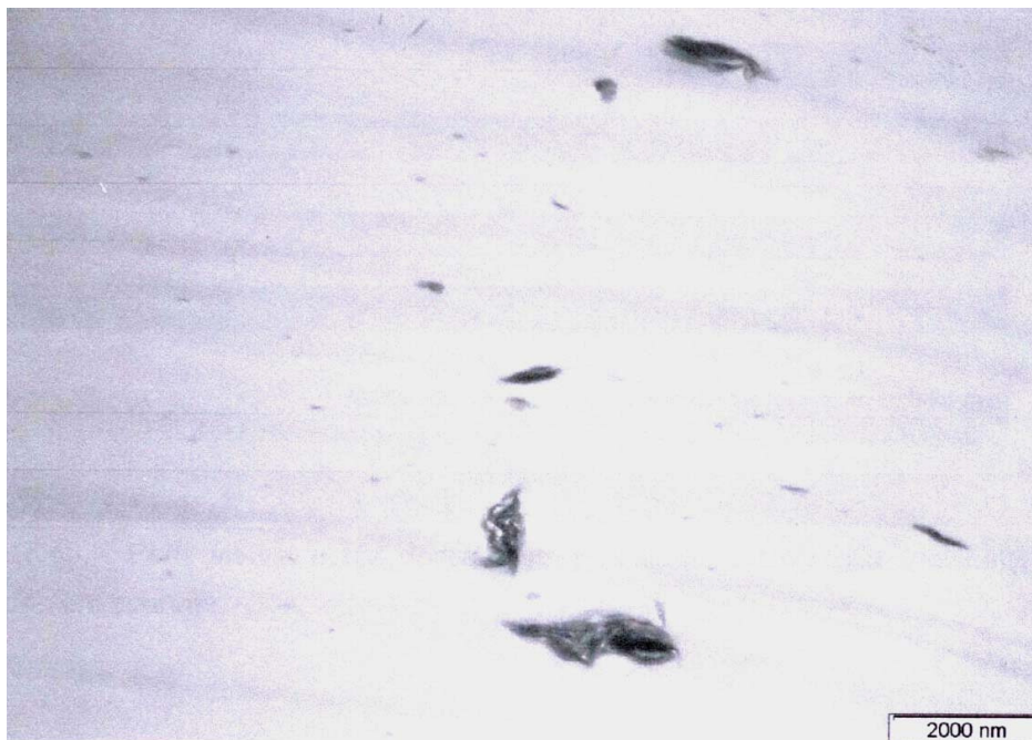
Figura 7.55 – PVC / 3% NanocorNa + (Extrusora Mono-Rosca – Com Tela)
