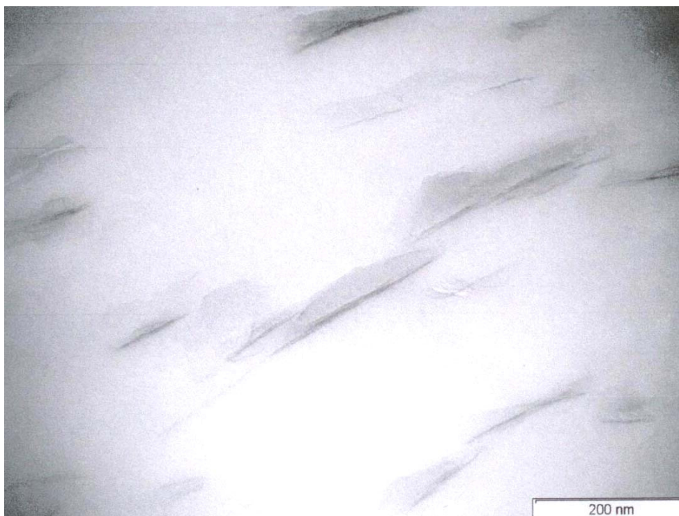
Figura 7.51 – PVC / 3% Cloisite 30B (Extrusora Mono-Rosca)
