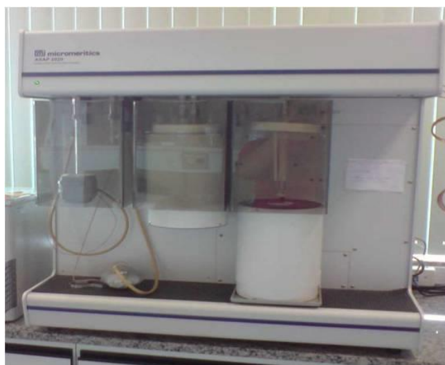
Figure 3.4 - Micrometrics equipment utilized for the measurement of BET specific surface area.
