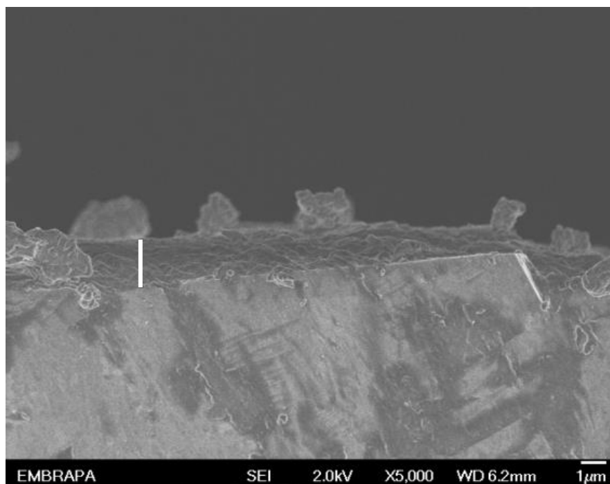
Figure 4.26 - Cross sectional FEG micrograph of SAM 1-ten layer \text{TiO}_2 film deposited on rutile substrate and calcined at 350\text{ }^\circ\text{C}/12\text{h} with a rate of 1^\circ\text{C}\cdot\text{min}^{-1}
