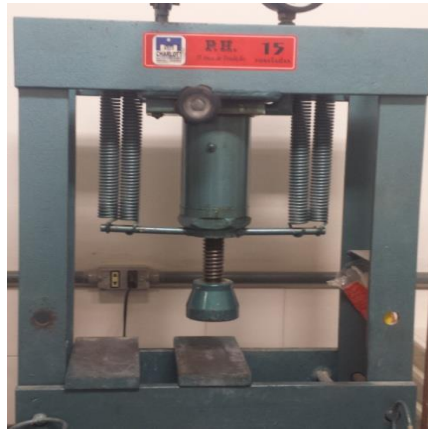
Figure 3.6 - Uniaxial pressing machine utilized for the compaction of the substrates.
