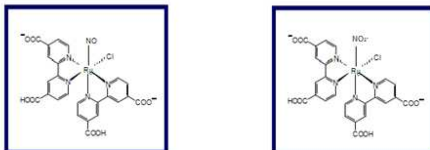
Figura 2. Estrutura dos compostos (a) cis -[Ru(H-dcbpy) - 2 (Cl)(NO)] e (b) cis -[Ru(H-dcbpy) - 2 (Cl)(NO 2 - )]
