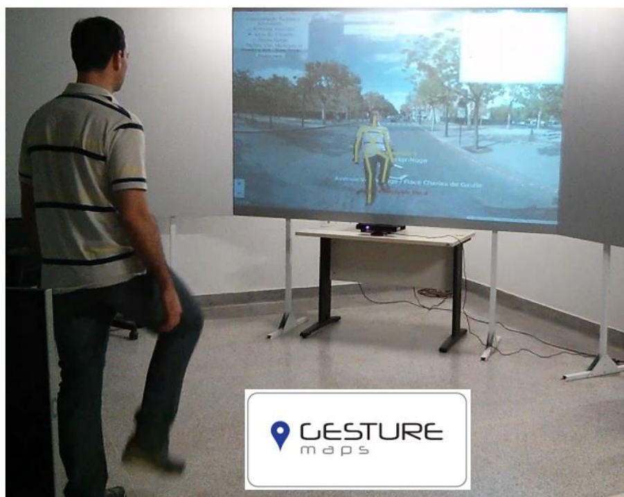
Figure 07: Subject using the GestureMaps application that can control Google Street View using legs' (lower limbs) movements.
