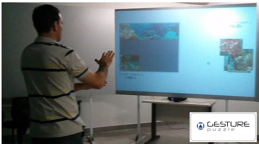
Figure 04: Example of subject playing GesturePuzzle, an application that can control a virtual puzzle using body gestures (upper limbs).
