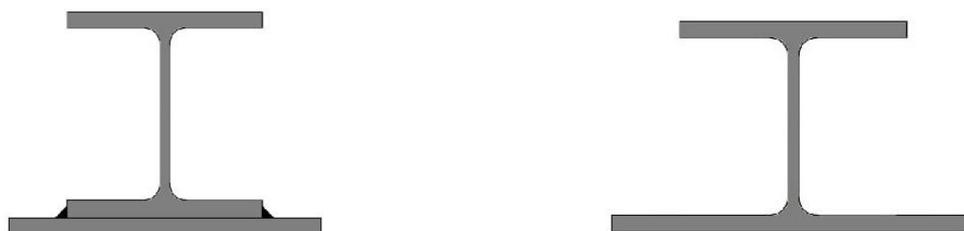
a) Perfil *Slimflor Fabricated Beam (SFB)*      b) Perfil *Asymmetric Slimflor Beam (ASB)*
