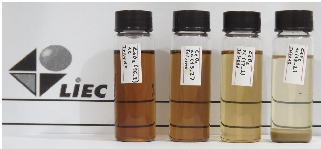
Figure 4.7 - Dispersion of the different synthesis made by the solvent-controlled method using previously dehydrated precursors; from left to right the samples has 0, 1, 3, and 5 mmol of OAm respectively
