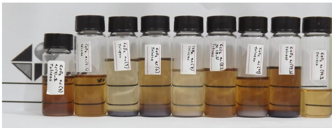
Figure 4.5 - Dispersions of the different syntheses made by the solvent-controlled method using hydrated precursors.
