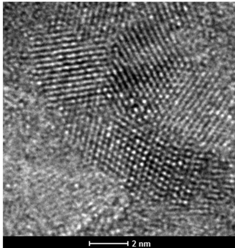
Figure 4.59 - HRTEM images of mixed nanoparticles ( \text{CeO}_2 and \text{ZrO}_2 ) after in situ heating at 950^\circ\text{C} for 360 minutes.
