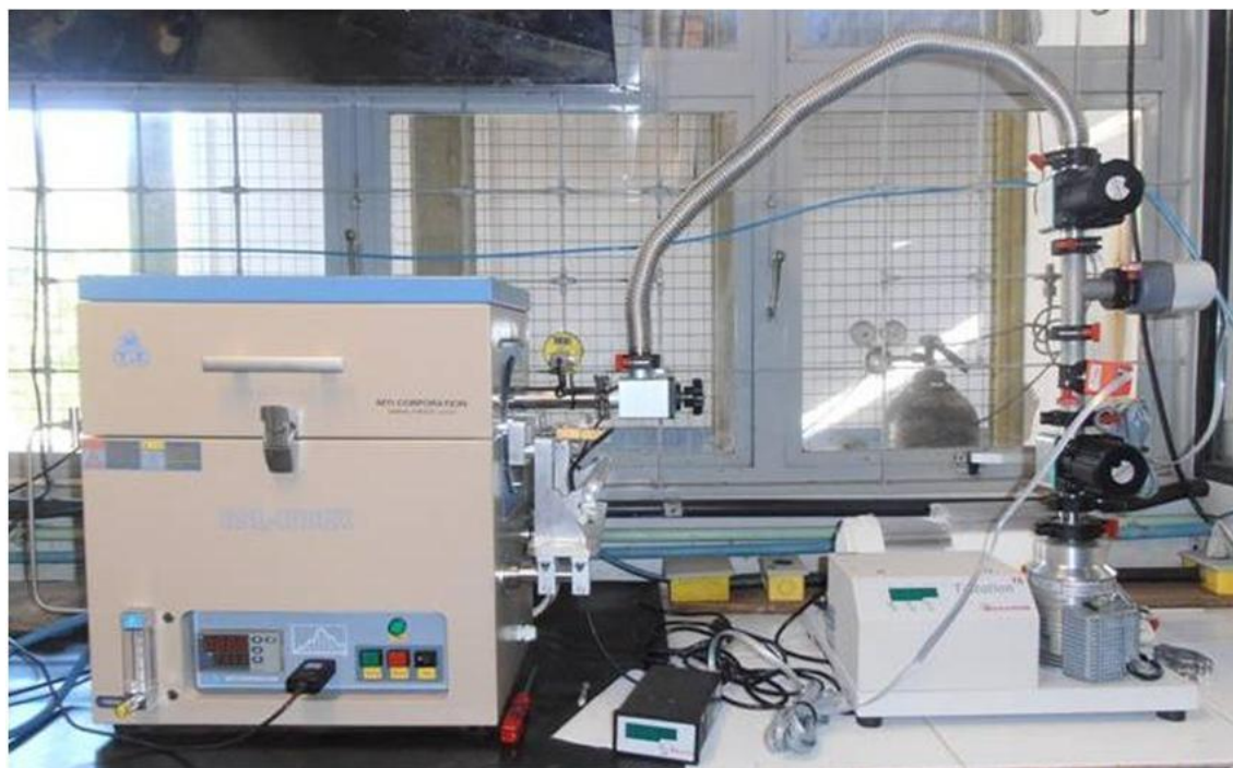
Figure 3.6 - MTI furnace with quartz tube, and T-Station 75D turbomolecular pump.
