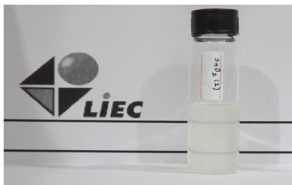
Figure A.2 - Dispersion of tin oxide nanoparticles synthesized by the solvothermal method.
