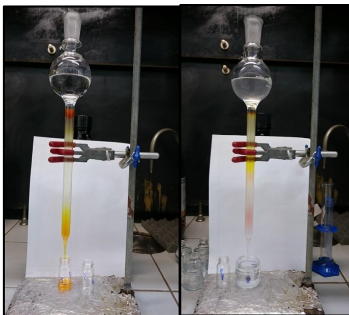
FIGURE 3.10 – Illustration of the chromatographic column performed on silica to the fraction PBCMe 03/07 col1.
