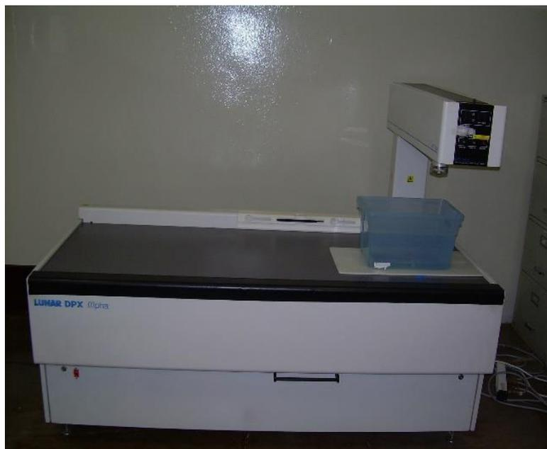
FIGURA 2. Densitômetro DPX-ALPHA.
