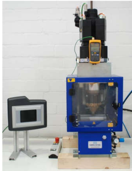
Figure 4.4 – Refill Friction Stir Spot welding RPS 100 (Hams & Wende) machine, developed by HZG and RIFTEC GmbH
