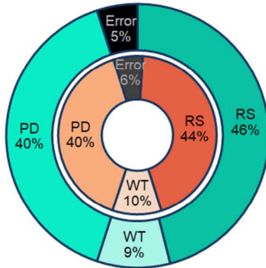
Figure 5.8 – Influence of individual parameters – rotational speed ( RS ), welding time ( WT ) and plunge depth ( PD ) – on the variance of LSS in terms of means (in teal) and SNR (in orange) given by ANOVA
