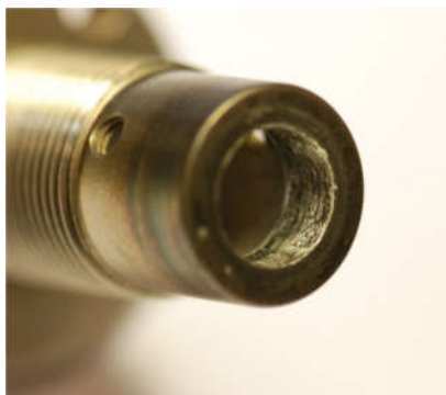
Figure 5.29 – Trapped aluminum on the clamping ring inner surface
