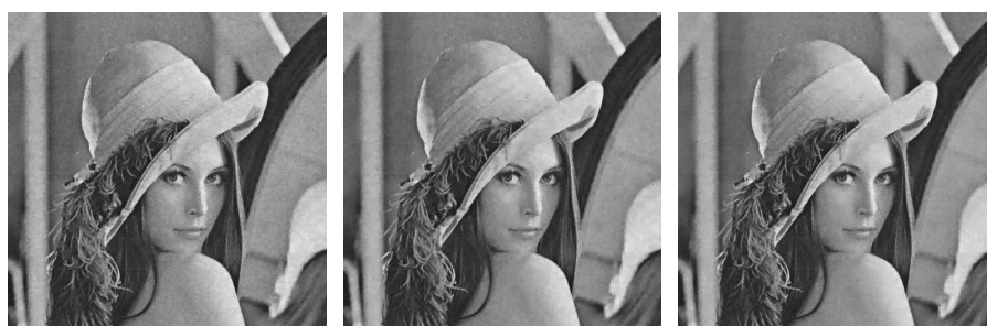
(e) Restaurada SDAE-KL PSNR:31,596 SSIM:0,913 (f) Restaurada SDAE-SSP PSNR:32,429 SSIM:0,932 (g) Restaurada MLP PSNR:32,391 SSIM:0,932
