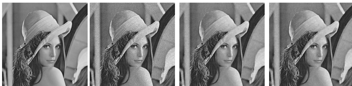
(a) Original (b) Ruidosa PSNR:22,931 SSIM:0,603 (c) Restaurada SDAE PSNR:32,326 SSIM:0,931 (d) Restaurada SDAE-FE PSNR:32,418 SSIM:0,932
