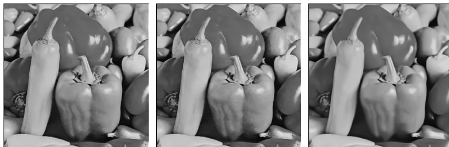
(e) Restaurada RDCNN-KL PSNR:36,277 SSIM:0,976 (f) Restaurada RDCNN-SSP PSNR:36,304 SSIM:0,976 (g) Restaurada BM3D PSNR:33,943 SSIM:0,908
