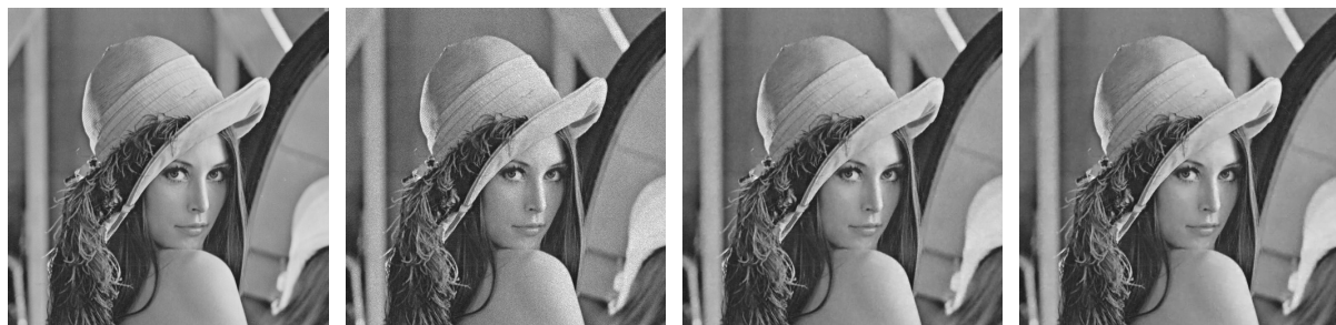
(a) Original (b) Ruidosa PSNR:30,291 (c) Restaurada SDAE PSNR:36,864 SSIM:0,970 (d) Restaurada SDAE-FE PSNR:37,061 SSIM:0,972
