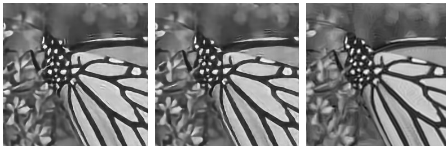
(e) Restaurada RDCNN-KL PSNR:24,802 SSIM:0,882 (f) Restaurada RDCNN-SSP PSNR:25,004 SSIM:0,883 (g) Restaurada DEBBM3D PSNR:25,881 SSIM:0,807
