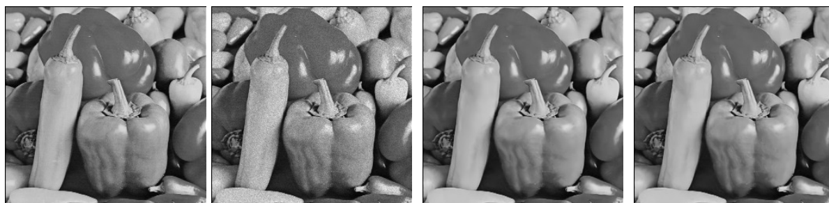
(a) Original (b) Ruidosa PSNR:30,153 SSIM:0,887 (c) Restaurada RDCNN PSNR:36,320 SSIM:0,976 (d) Restaurada RDCNN-FE PSNR:36,253 SSIM:0,976
