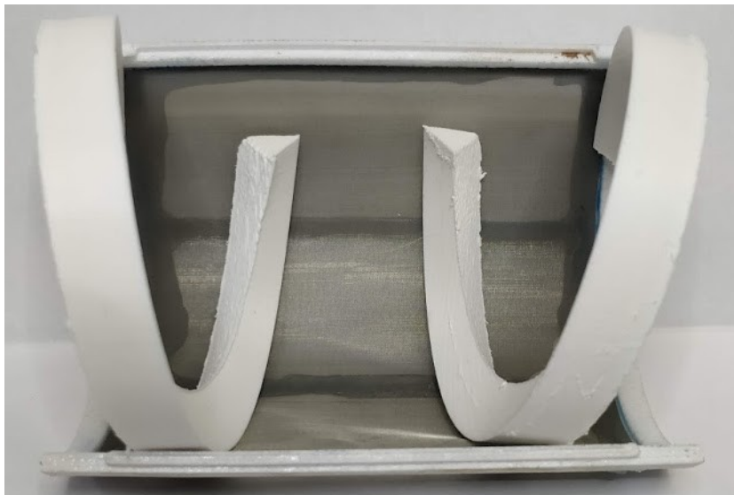
Figure 7.8 Horizontal Reactor with Screw Baffle – Mid Section Cut
