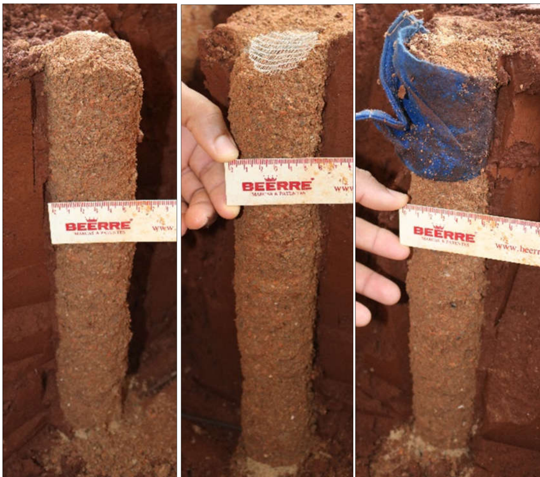
Figura 48 – Exumação das colunas: (a) RCC; (b) RCC + GGH; (c) RCC + GTNT Enc. (a) (b) (c)
