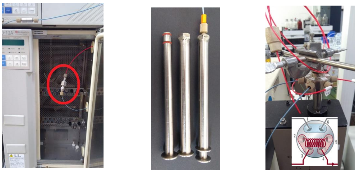
Figure 4. Open oven with the reactor inside (Left). Syringes (middle). Injection Valve (Right).
