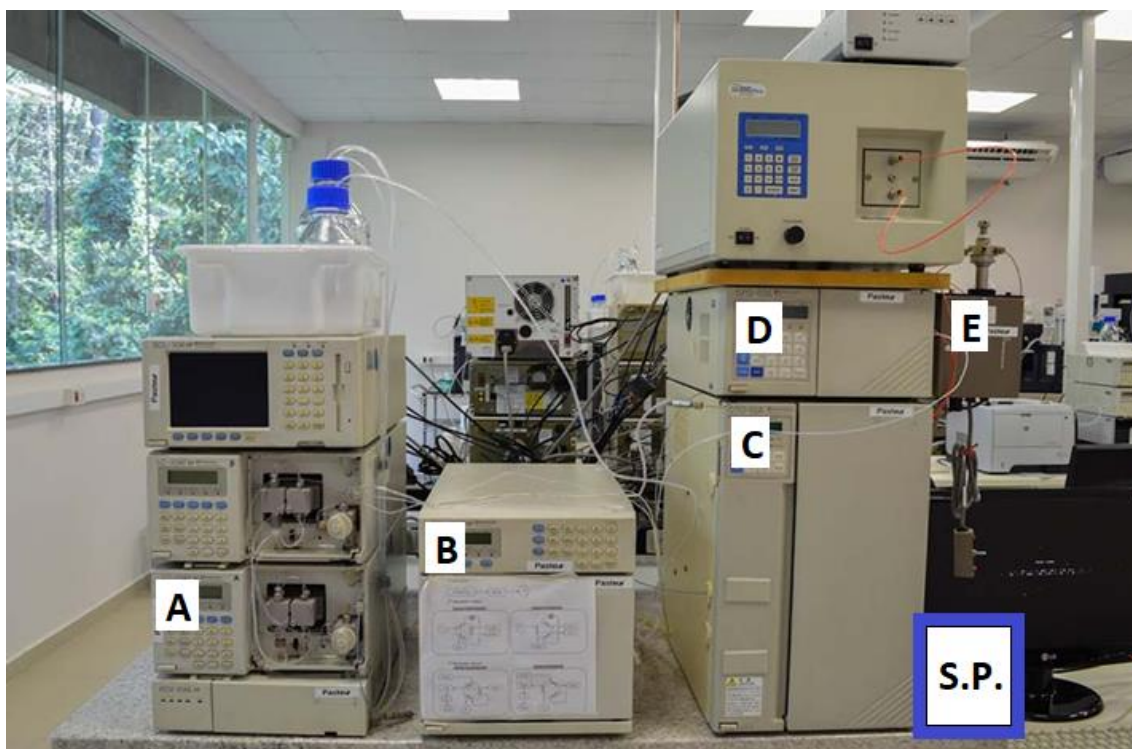
Figure 3. Reactional flow system for the simultaneous production and analysis of Triazoles. A-Pump, B-Auto Sample, C-Oven, D-UV-Vis Detector, E-Injection Valve, S.P.- Syringe Pump.
