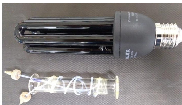
Scheme 32. Internal Photochemical Reactor Setup
