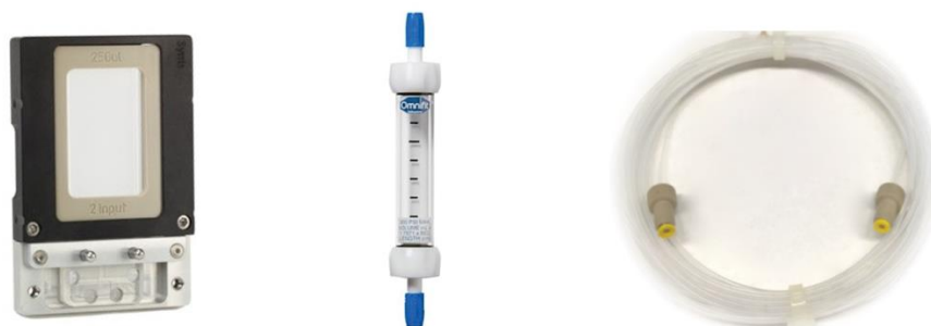
Scheme 22. Transparent flow reactors: chip, column (middle), tubular (right).
