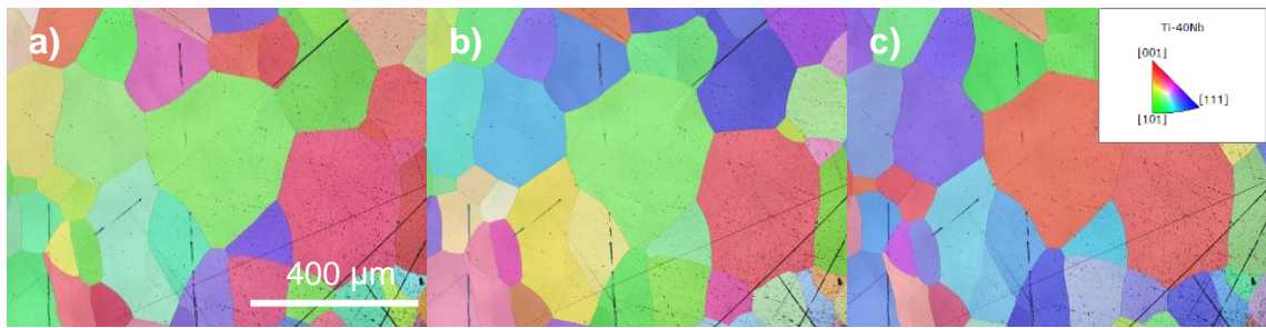
Figure 4.8. Electron back-scattered diffraction maps of a suction-casted sample of the TNZT alloy submitted to homogenization heat-treatment: Inverse-pole figure (IPF) in the x- (a), y- (b) and z- (c) axis. The inset is the IPF orientation reference.
