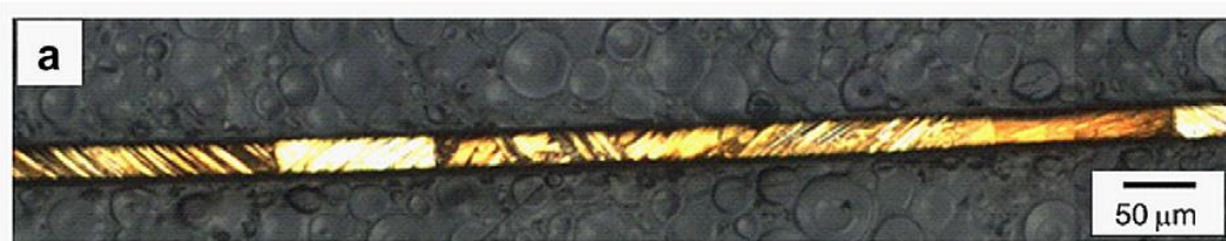
Figure 1.3 Optical micrograph of a Cu-Zn-Al microwire longitudinal cross section, with bamboo-like structure of grains [34].
