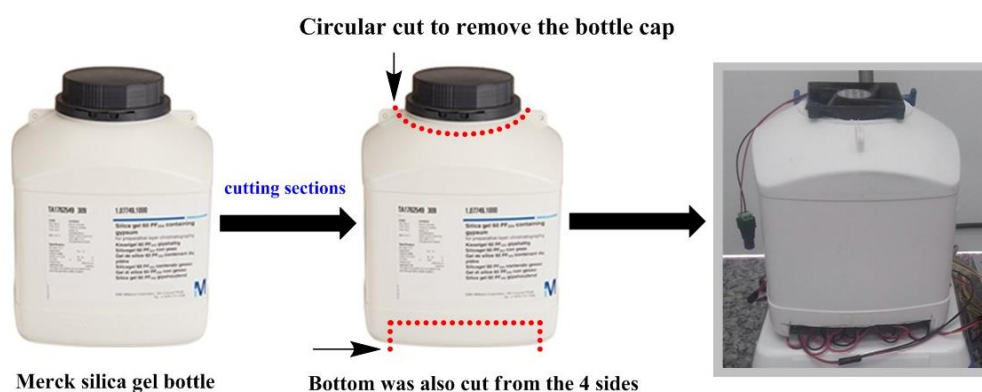
Figure 10. Silica gel bottle used as the reactor body.
