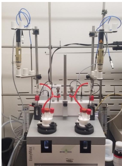
Figure 29. EasyMax 102 from Mettler Toledo used to carry out batch experiments.
