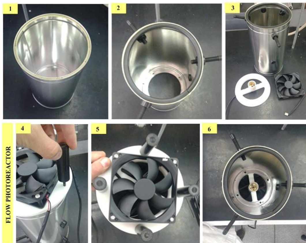
Figure 14. Construction of photochemical reactor for continuous flow reactions.
