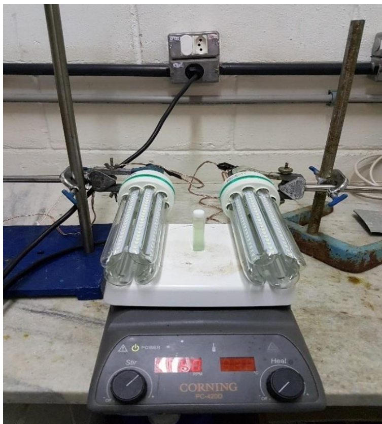
Figure 1.14 – Experimental setup used in the photobleaching studies.
