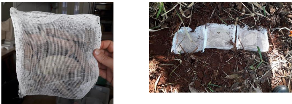
Figure 6 (On the left) Example of litter bag assembled with leaves mixed from all four plots of area R1. (On the right) Row of litter bags from areas R1, R2 and R3 getting buried underground.
