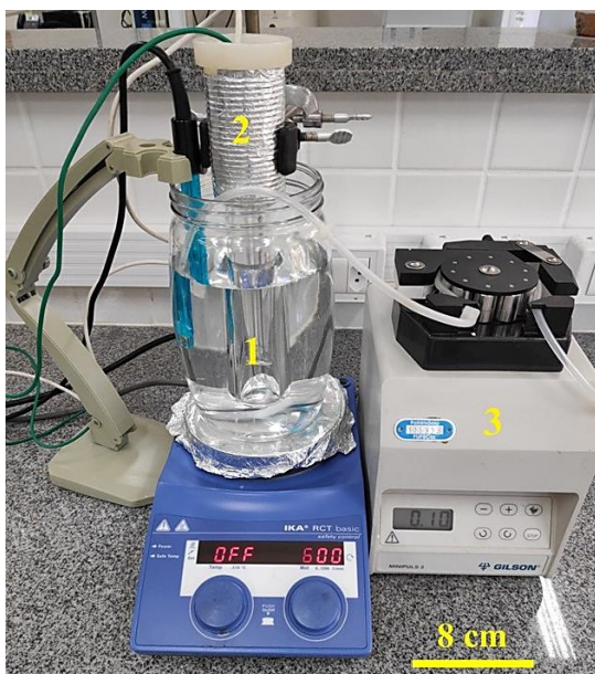
FIGURE 2.1 – Image of the experimental setup used during the degradation and mineralization of BPA solutions through different UVC AOPs: reservoir (1), quartz tube with the UVC lamp inside it (2), and peristaltic pump (3).
