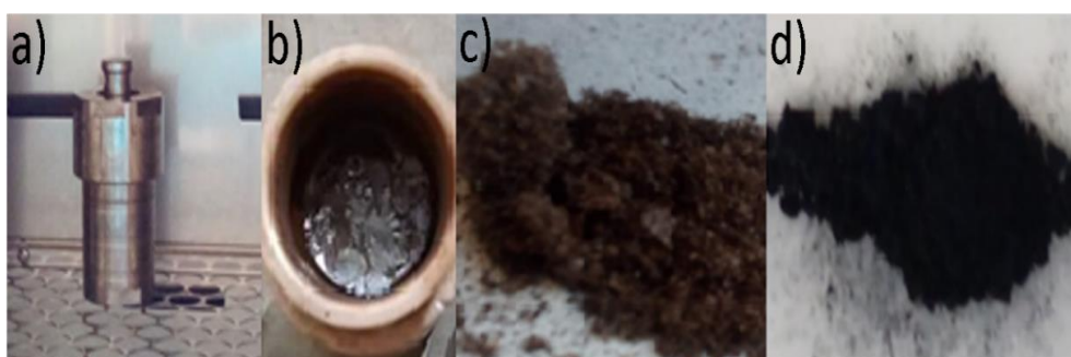
Figure 3.10- Schematic representation of hydrothermal synthesis of boron-doped carbon samples. a) Sucrose and Boric acid were dispersed in water, followed by hydrothermal synthesis in autoclave and, b, c) the product collected, washed, dried, and d) carbonized, resulting in boron-doped carbon.
