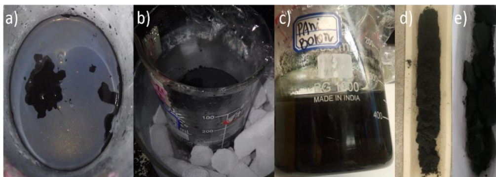
Figure 3.11- Preparation of the sample constituted by nitrogen-boron co-doped carbon material. a) Dispersion of boron doped carbon BC-900 into water, b) boron doped carbon, aniline monomers and acid dispersed in beaker and placed in cold bath, c) PANI coated onto boron doped carbon, d) Dark green colored PANI coated boron doped carbon, and e) Boron and nitrogen co doped carbon after carbonization.
