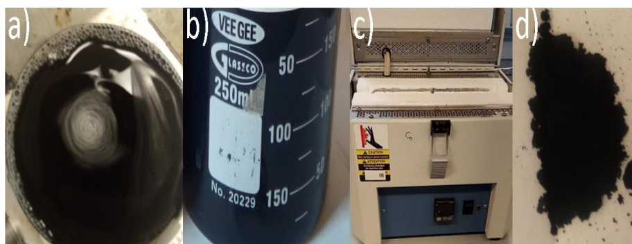
Figure 3.4 - Synthesis steps for preparation of sulfur-nitrogen co-doped carbon, a) Nitrogen-doped carbon is dispersed in solution with emulsifier, followed by addition of oxidizer, b) Polymerization of PEDOT onto nitrogen doped carbon coated \text{Si}_4\text{N}_3 , c) Carbonization of material in furnace, and d) Nitrogen-sulfur doped carbon.
