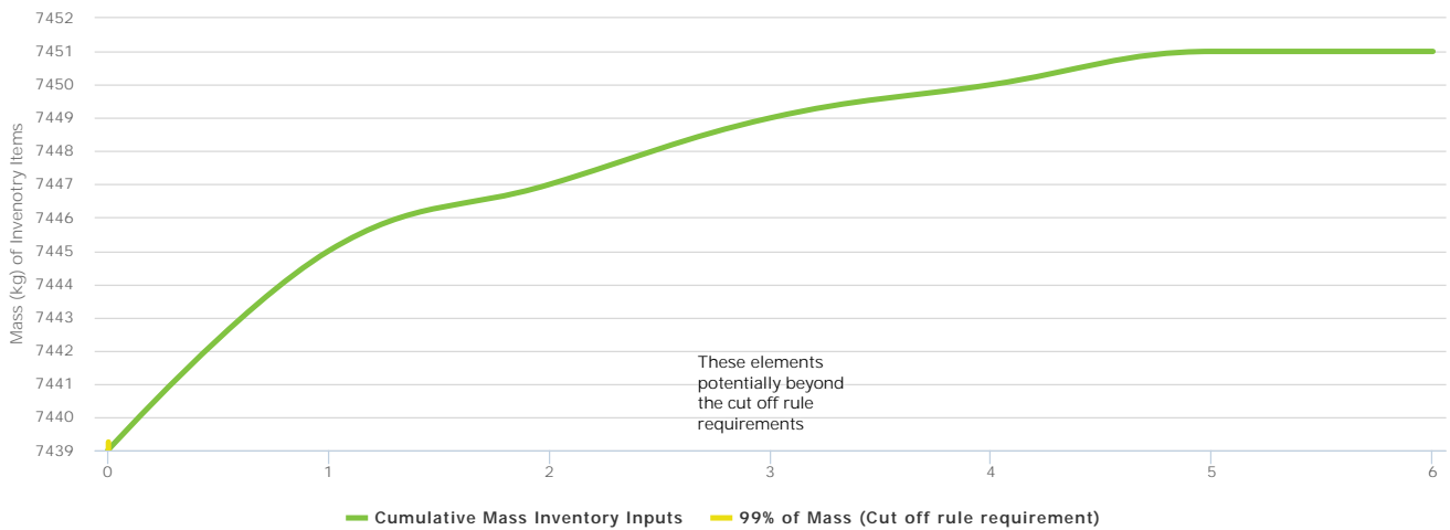
Figure 5: Cumulative Mass Inventory Entries. In this case 85.71% make up the last 5% of mass inventory entries.
