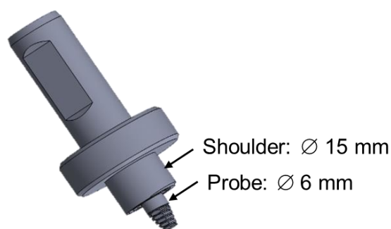
Figure 4.1 – Tool attachment configuration used for welding.
