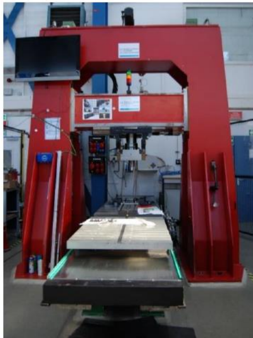
Figure 4.2 – Gantry System – Friction Stir Welding machine.
