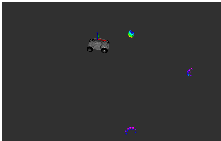
Figure 3.3 – Simulation test for the cloud downsampled with PassThrough and CropBox filters
