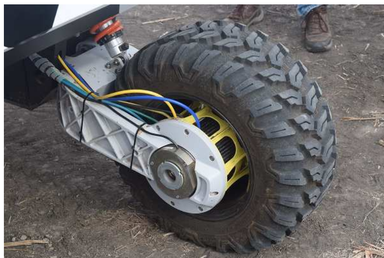
Figure 11: Suspension of the Agbott II [20]
