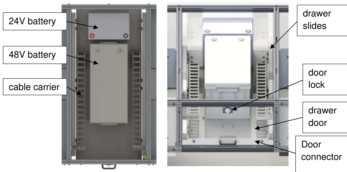
Figure 33: (a) Top view drawer, (b) 3D-view drawer
