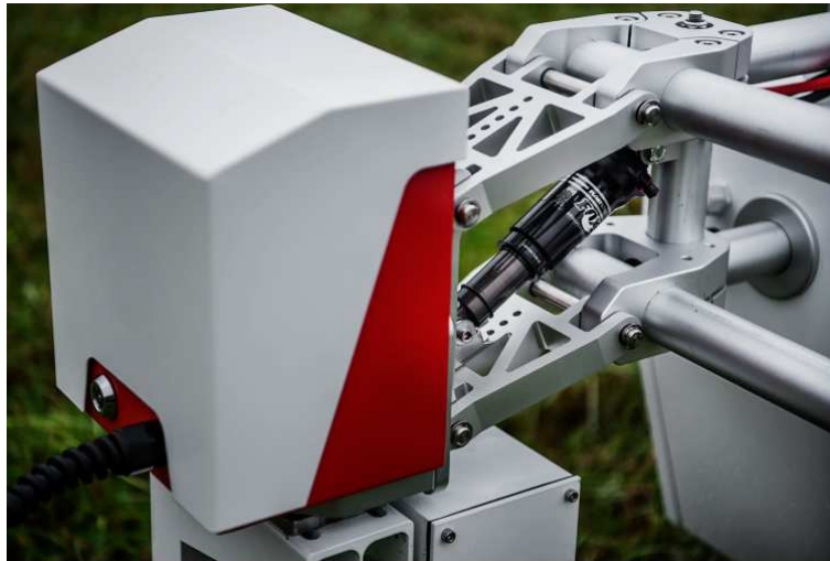
Figure 10: Saga Robotics' Thorvald II AGV suspension [19]
