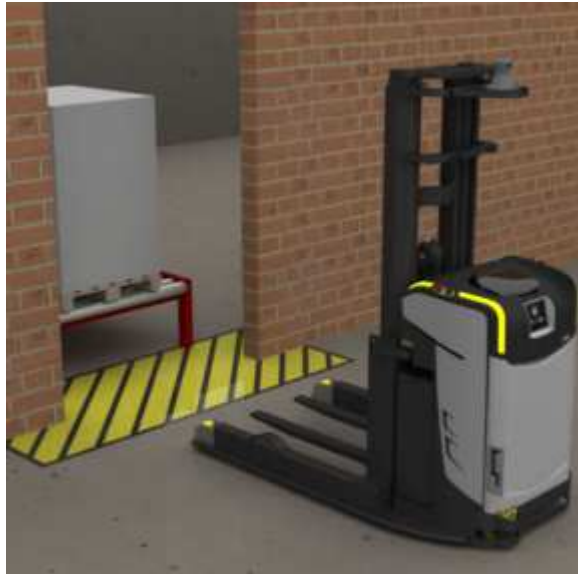
Figure 62: Hazard zone marked on the floor [40]
