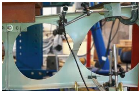
(b) Web post buckling phenomena [14] (with permission from Elsevier)
