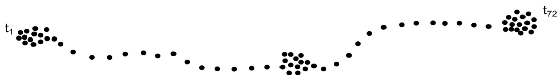
Figure 1.1 – Example of a raw trajectory obtained by sampling a user's geo-location at different timestamps. Each black dot represents a sample, and their clusters show locations where the user stayed for a while. Source: Ferrero et al. (2020) .
