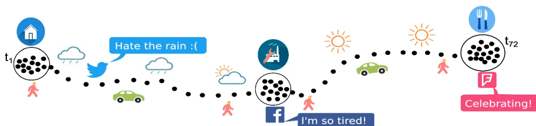
Figure 1.2 – Example of a semantic trajectory obtained by processing data from Figure 1.1 and integrating it with external sources. Data such as weather, social media messages, transportation means and place identification help to capture the context in which the trajectory occurred. Source: Ferrero et al. (2020).
