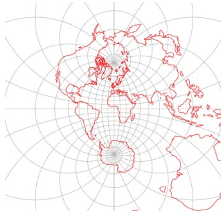
Figure 2.4: Stereographic projection applied to Earth [1].
