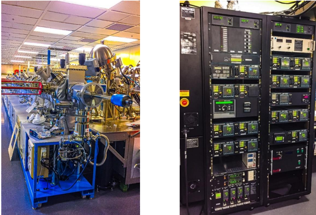
Figure 18 - Photos of the MBE system: growth chambers (left) and power controller (right).
