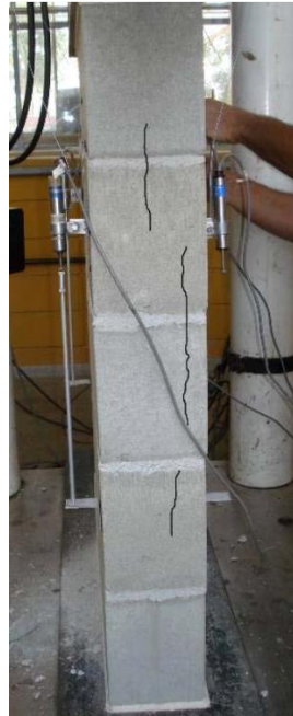
(a) Argamassamento total
