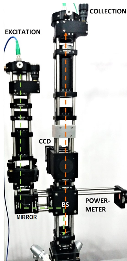
Figure 3.9: Photograph of the head of the confocal microscope with the main optical components and the different light paths. The green dashed line represent the excitation path and the red dashed line with arrow represent the detection path that is sent into one of the detection fiber.
