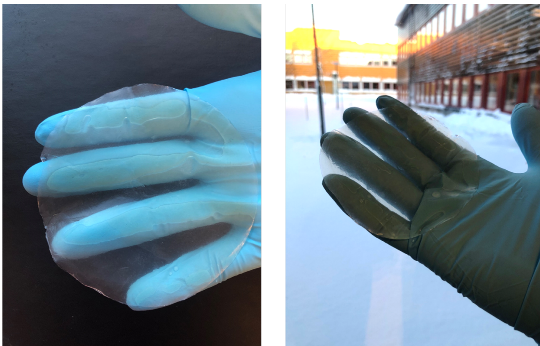
Figure 4.11. Photographs of the T-GNF hydrogels at 40 g/m 2 after reaching the equilibrium state.
