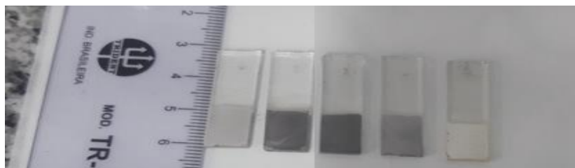
Figure 3.10 - Photograph of the films deposited by electrophoresis. Left to right (5Ti-40Ti_W).
