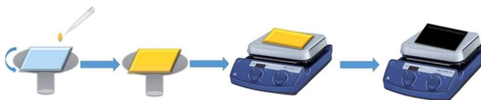
Figure 3.5 - Sequence of film deposition by the one-step method (1000 rpm/30 s and temperature 150 °C /10 min) [207].
