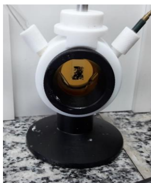
Figure 4.29 - Photograph of degradation of \text{MASnI}_3 electrode in 0.1 M tetrabutylammonium hexafluorophosphate (dichloromethane).
