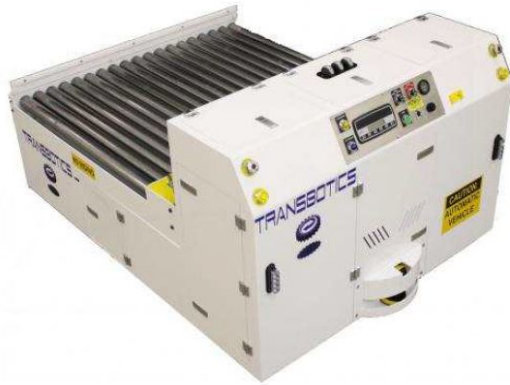
(a) Unit load AGV model.
