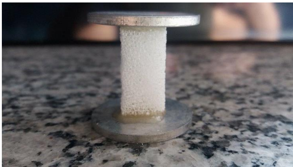
Figure 4.11 - Image showing the arrangement of the scaffolds for mechanical tests.
