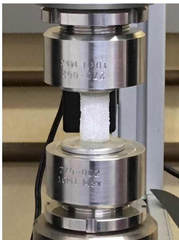
Figure 3.3 - Mechanical testing system (Instron-4467 model).
