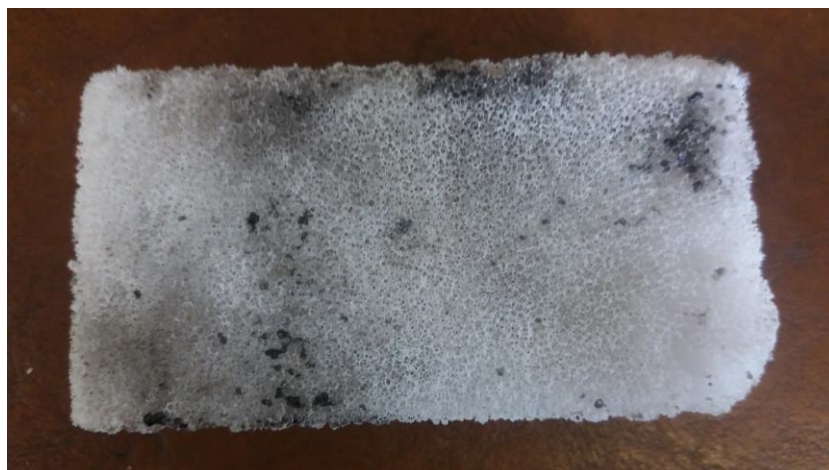
Figure 4.27 - Image of F18 glass-coated 590RP.BioS scaffold after heat treatment. PU foam size used as polymer template was 80x50x30 mm 3 .
