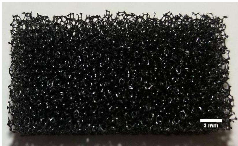
Figure 4.6 - The 860-PU foam cut in a square prism shape, with 15 x 15 mm 2 square base and 30 mm length to synthesize F18-860SP.BioS scaffolds.
