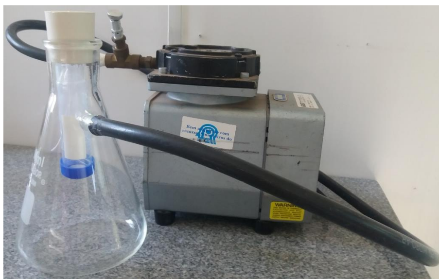
Figure 3.1 - Image of the system used to do vacuum and force the slurry gets inside the porous walls. This system was used to carry out the preliminary tests.
