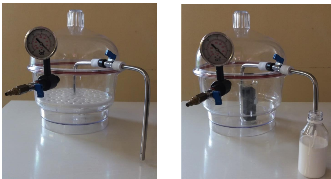
Figure 3.2 - Vacuum system to infiltrate scaffolds during second, third, fourth, fifth and sixth dipping.
